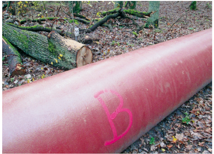
Figure 9: After the oak had been removed there was no sign of damage or even any alteration in the coating
