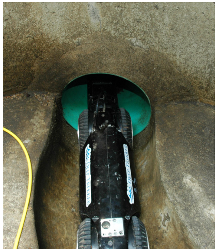
Adopted for use in potable and wastewater inspections: deploying the portable DT340 pipe crawler into a storm pipe
