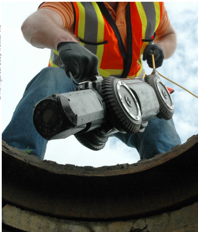
Adopted for use in potable and wastewater inspections: deploying the portable DT340 pipe crawler into a storm pipe
